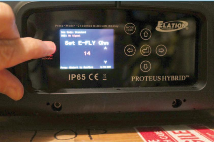
The Proteus Hybrid includes Elation's E-Fly wireless DMX transceiver.
