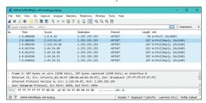
In the example above, you can see that there is Art-Net communication on a number of IP addresses. Try browsing to each one in turn to locate the lost device.
